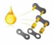
The lubricant's most important task is to lubricate the shaft and sleeve in the link. If there are an excess of liquid, this will not collect dust and other particles in the same way as usually happens.
